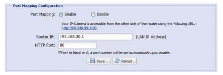
**Note:** When the configurations are saved successfully, you'll see a message indicating the IP address and port number assigned to this camera.
