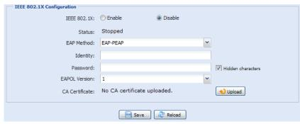
Step5: Disconnect the camera from your PC or laptop, and connect it to the switch in the LAN environment you want to use IEEE 802.1x, and the camera will start the authentication later.
